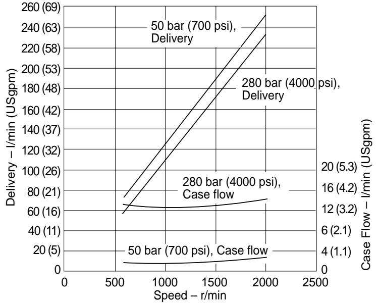
Delivery and Case Flow Versus Speed @ 93°C (200°F), full flow and 1.0 bar absolute (0 psi) gauge Inlet
